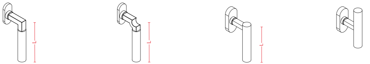
750310XX L 114 mm ON ROSE L 26 mm H 65 mm T 11 mm KEY 7 mm 770310XX L 122 mm ON ROSE L 26 mm H 65 mm T 11 mm KEY 7 mm 750332XX L 80 mm ON ROSE L 26 mm H 65 mm KEY 7 mm 750331XX L 80 mm ON ROSE L 26 mm H 65 mm KEY 7 mm
