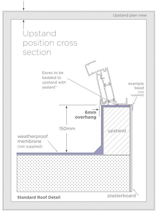
\*Sealant to be applied to the underside of the eaves as per installation guide instructions only
